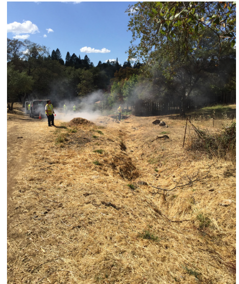
Smoke Test for Leachfield Capacity Evaluation
