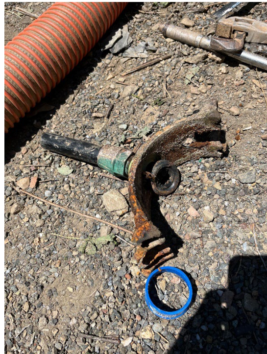
Saddle/Service Line Replacement – 24 Labor Hours | Excavator, Vac Trailer, Service Truck
