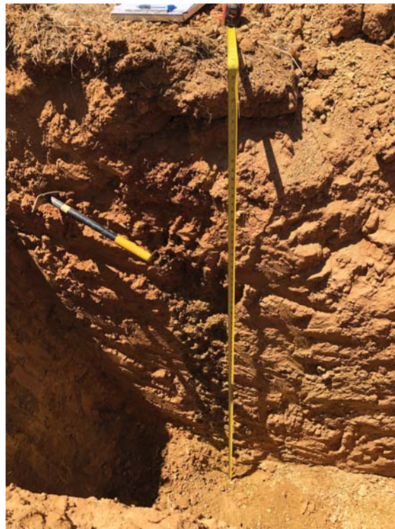
Photo No. 20 Soil profile in Test Pit TP9 (photo date 8/6/2020).
